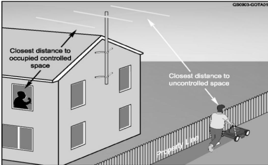
Figure 1 — Geometry of distances to consider for evaluation of maximum permissible exposure.
